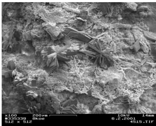
Fig. 2. Encrustation is marked on ofloxacin blended coating. Magnification: 100×
